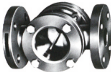
MODEL NO.:FITZER / SFI / 801 Flapper type Sight flow indicators are best suited for horizontal flow OR vertically up ward flow The position of flapper gives an indication of the flow passing.
